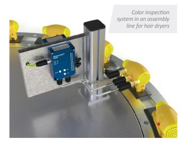
controller (Siemens S7). The color values are checked for plausibility during a so-called recipe management, where upcoming errors are detected. By standardizing the transmission, the data integration of the sensors is accomplished within no time. In addition to the color values, status information and a live counter can be evaluated. The live counter signals that the respective sensor is still working properly.
